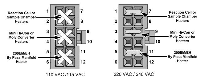
Figure 2-4: Typical Set Up of AC Heater Jumper Set (JP2)
